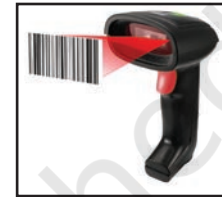
Figure 1.12: Capturing data using barcode reader
